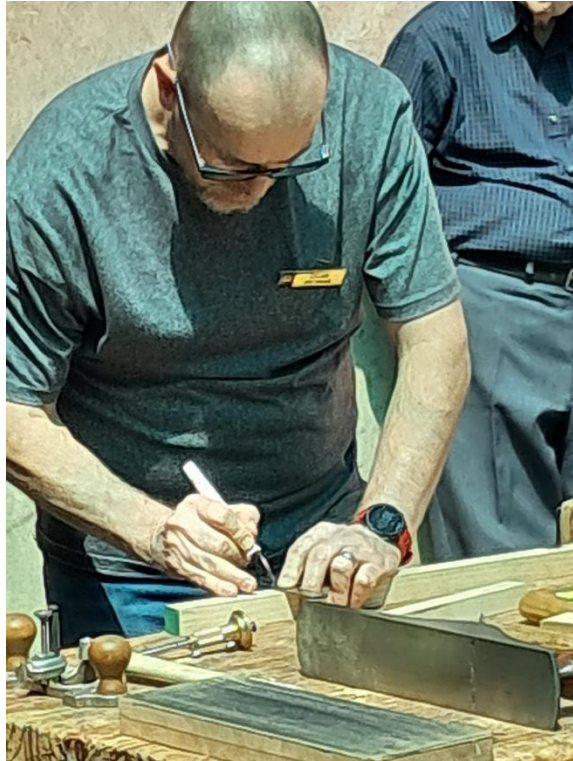
Dylan using a marking knife to ensure accurate joinery
